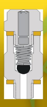
A check valve inside of the nozzle prevents it from dripping,
